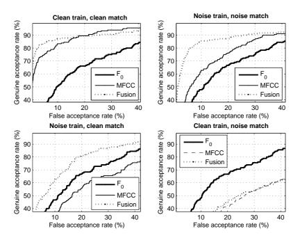
Figure 3: ROC curves of  $F_0$ , MFCC and their combination in different conditions.
